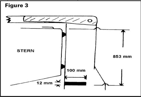
**5.14.4** When in sailing trim (without crew) with all supplies, sails, stores, tankage, and sailing gear, the bottom of both lines should touch the water.
